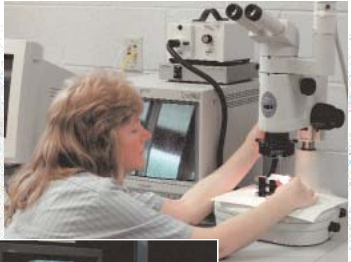
The stereo microscope shown here is particularly useful in contamination testing to identify its origin.
