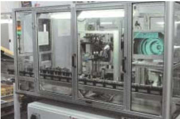
Fully automated assembly line producing 2 million parts per year confirms a "passed" assembly with in-process part presence camera.
