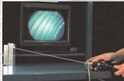
Borescope being used for internal inspection of a manifold which HUSCO supplies with four valves and a filter as a complete assembly.
