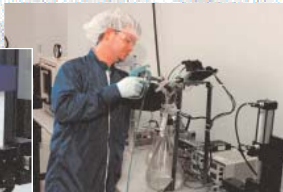
Regularly scheduled cleanliness testing performed in a clean room environment. Analysis for contamination size, weight and material are performed in-house.
