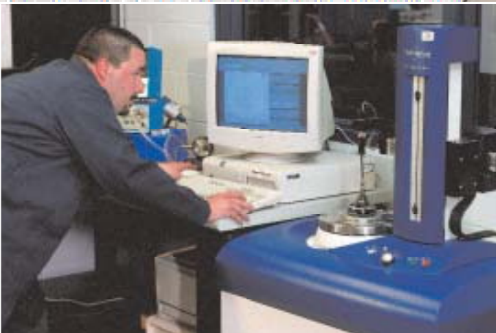
Quality technician using a Talyrond to precisely measure roundness, straightness and cylindricity at incoming inspection.
