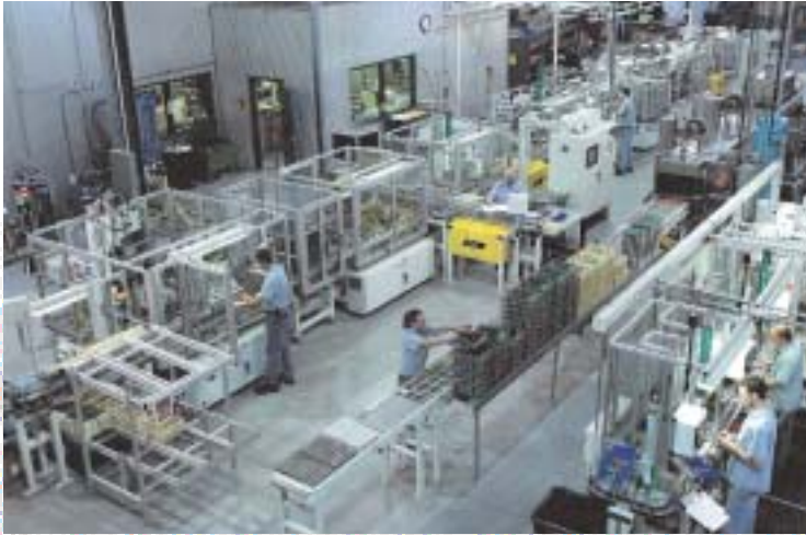
Automated wash line feeding multiple production cells.
